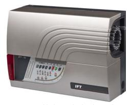
ICAM IFT-15 detectors are multi-channel microbore air-sampling systems with an alarm sensitivity range from 0.001% to 20% obscuration/m (0.0003% to 6.10% obscuration/ft). These detectors are classified as a Very Early Warning Smoke Detectors and can reliably detect fire at an early stage, and low to high concentrations of smoke. As a multi-channel system, the IFT detector is able to divide a protected space into sampling sectors, enabling the localization of a fire for faster incident response.
